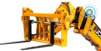
The boom on a Construction Loadall is mounted low in the one-piece fully welded chassis, providing a very rigid structure and maximum over-theshoulder visibility. We've fitted a tough inverted U-shaped boom pressing with fully welded closing plates. For extra strength, we've reduced the number of joints and stress points across our integrated boom nose and one-piece closing plate.
