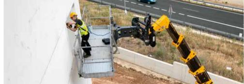
Further widening the versatility of the JCB Loadall, the aerial work platform is more mobile and cost effective than a boom or scissor lift.
