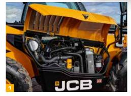
By producing high levels of power and torque even at engine speeds as low as 1300– 1400rpm, the Dieselmax engine can provide fuel-efficient matching of transmission and hydraulics.
