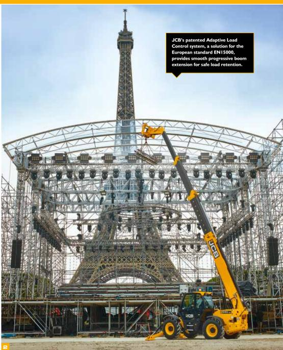
With a 10% reduced turning circle than the 540-170 as well as 1000kg lighter thanks to a shortened chassis and lightweight boom sections, the 540-180 HiViz is one of the most manoeuvrable machines around.
